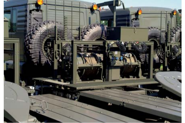
Heavy load truck with Rotzler HZ 200 double-winch systems (pulling force: 2 x 200 kN)
