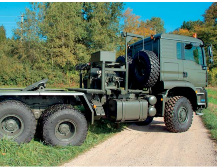
A spare wheel holder for two spare wheels is situated between the driver's cabin and the double-winch aggregate
