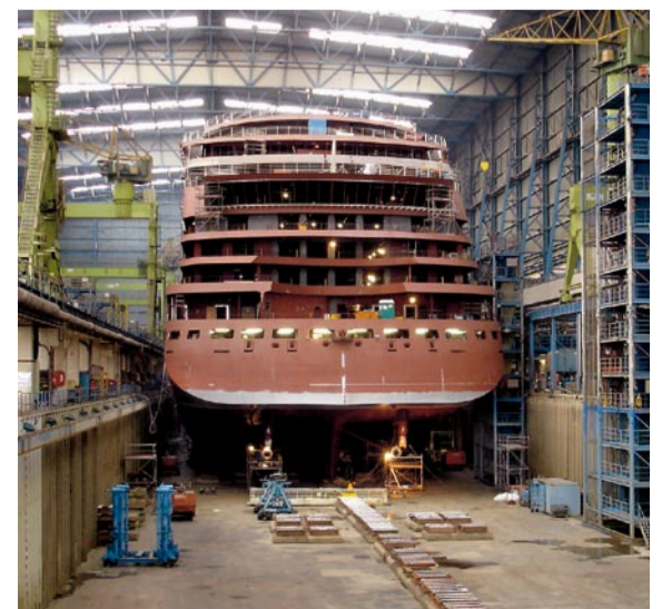
Honeycomb-style integration of the passenger cabins into the hull
